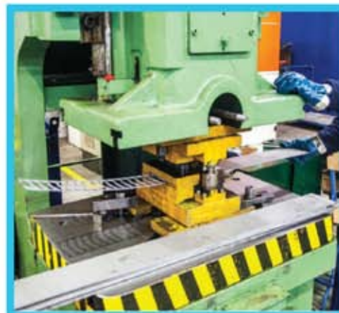
Installation: Mechanical Power Press
