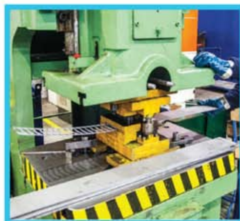
Installation: Mechanical Power Press
